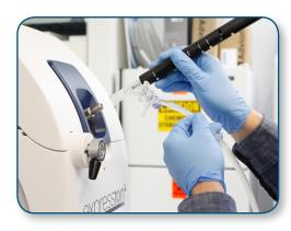
The apparatus consists of an extended ASAP probe protected in an exterior sheath fitted with a three-way valve allowing the system to be flushed with inert gas and then sealed. In this manner it is possible sample a reaction mixture on the iASAP probe, seal it in inert gas and then take it to the mass spectrometer for analysis.
